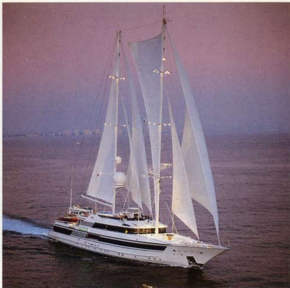
With her tandem centreboards and efficient rig, The Other Woman is stiff (less than 10° of heel) and promises both a fast pace and comfort for passengers under sail
